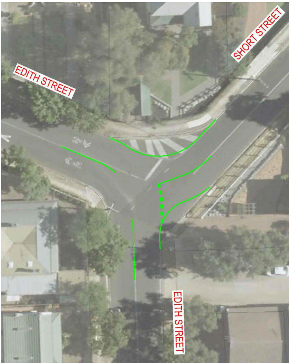
Figure 17: Recommended realignment of Edith Street/Short Street intersection
