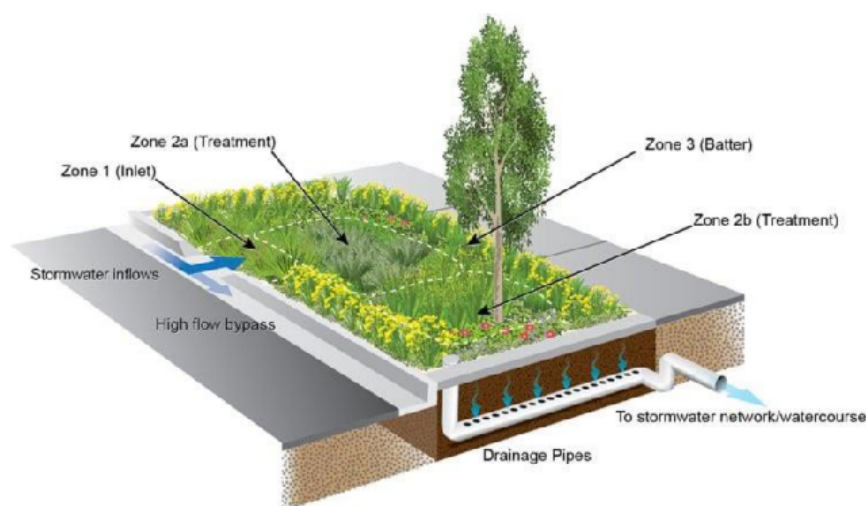
Figure 5.17 Typical layout of a raingarden (Water Sensitive SA)
