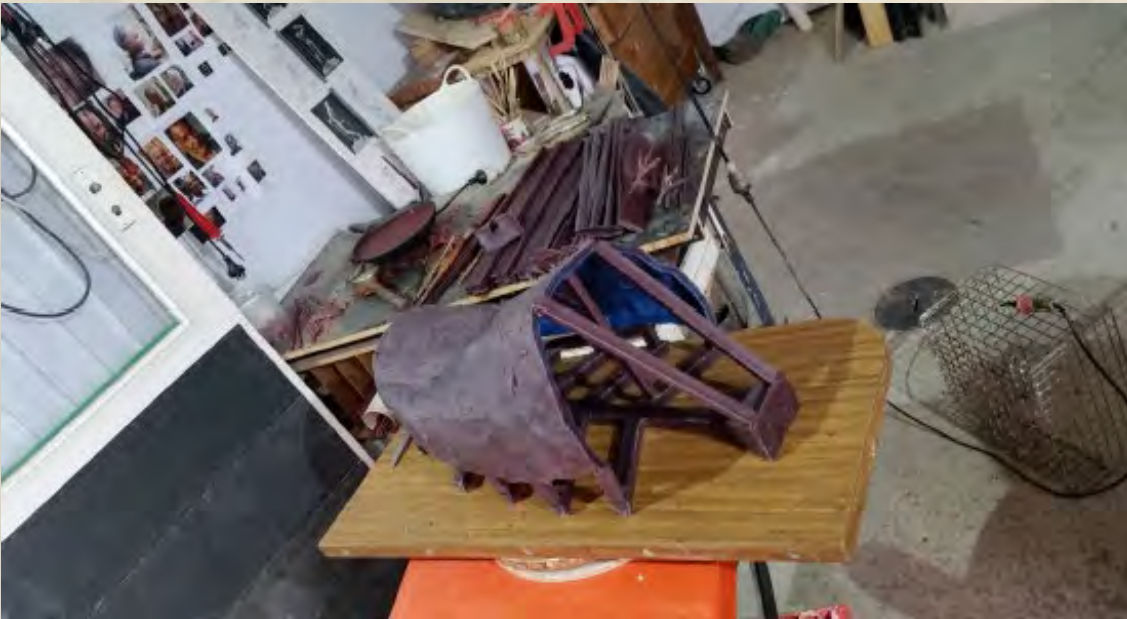
The wax section with its feed system attached all constructed in wax.
