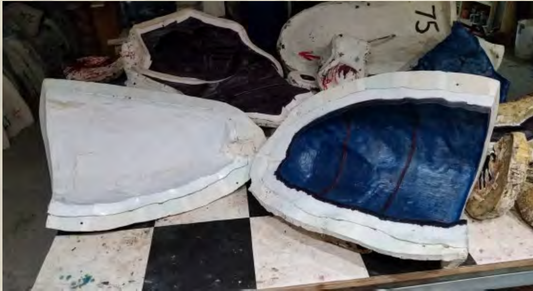
A mould section with wax painted into it – 4mm in thickness.
