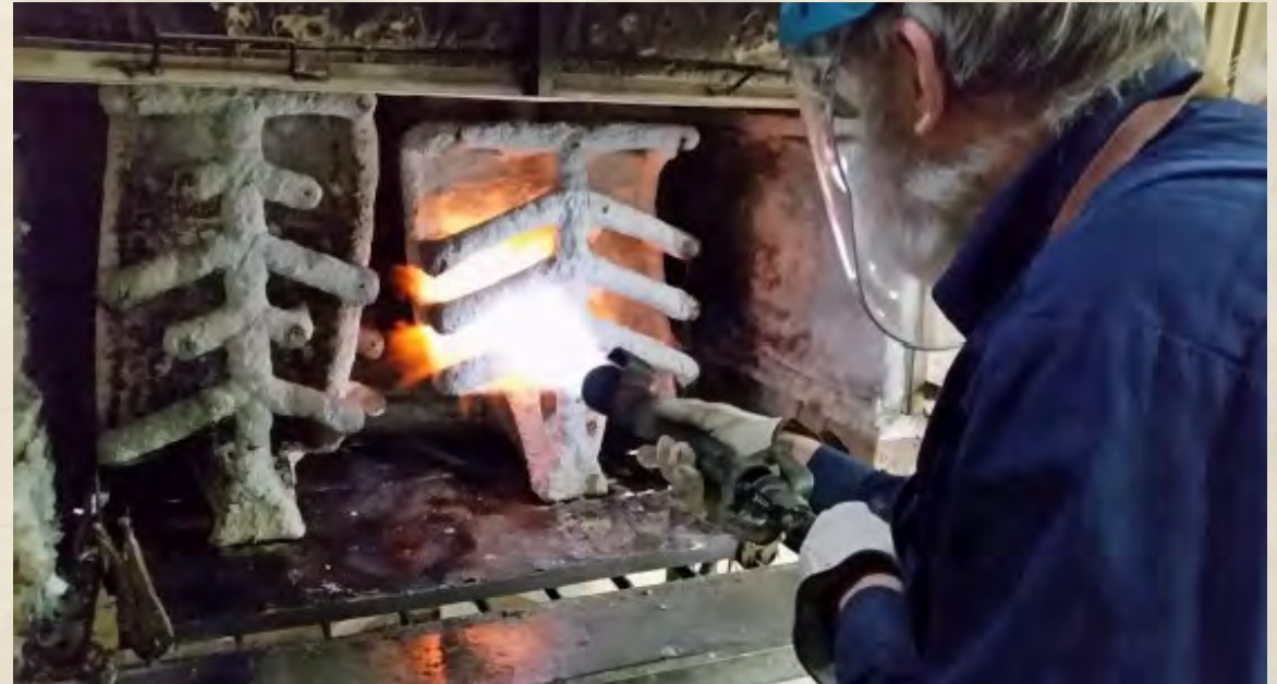
Removing the wax from the heatproof moulds.
