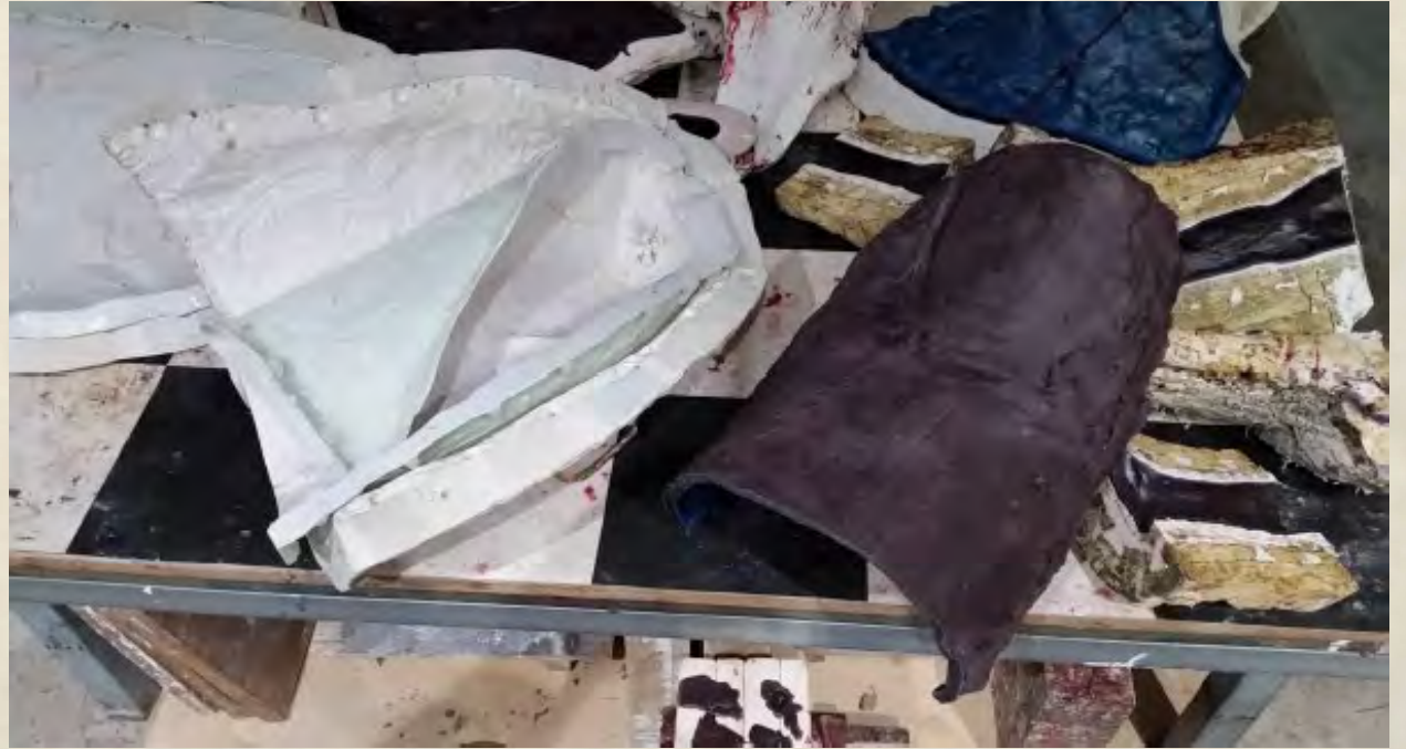
A wax section sitting next to the plaster and silicone rubber mould.
