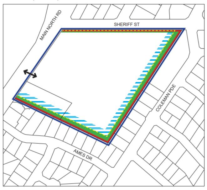
Concept Plan Boundary No vehicle access Landscaping (minimum depth of 1.5 metres) Landscaping (minimum depth of 3 metres) Acoustic barrier
