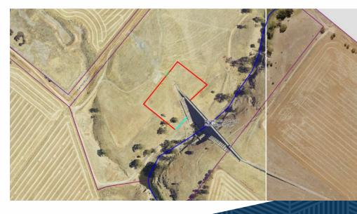
The red line indicates the existing fence which is in good condition. The blue line shows the section where fencing is required to be installed and the small green line is the current access gate.
