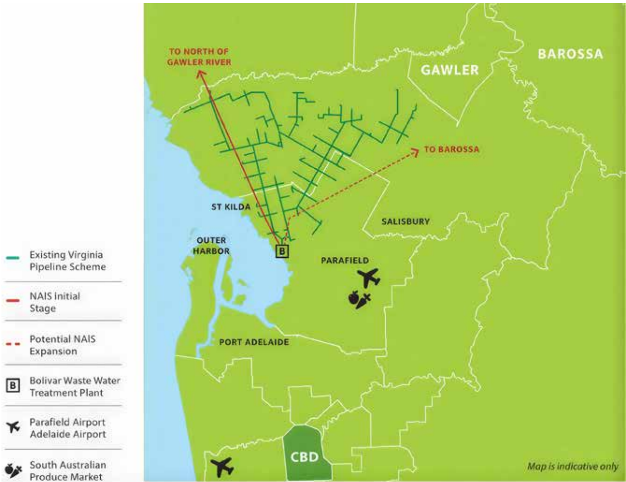
Figure 10. A number of recycled water schemes operate within the northern growth corridor sourced from Bolivar treatment plant, including the Virginia Pipeline Scheme and the Northern Adelaide Irrigation Scheme (Source:6.-NAIS_Information-brochure.pdf)
